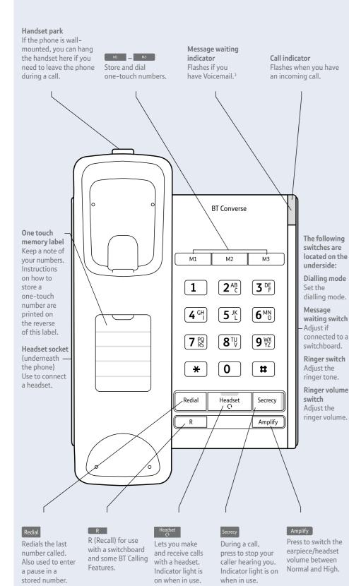
1 The light will only flash when connected to a PBX switch or similar.
